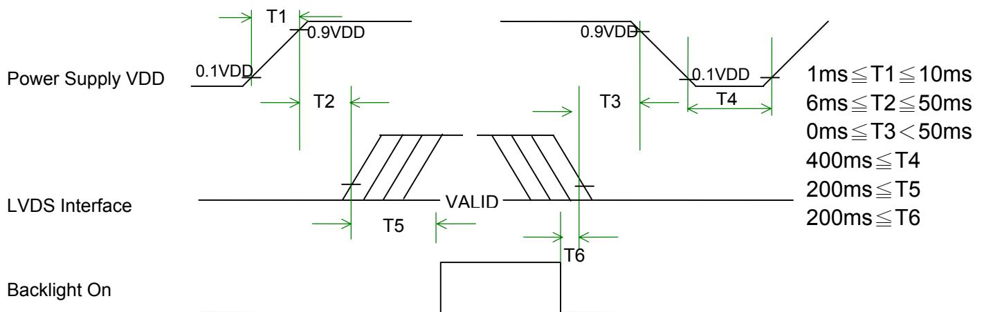
Apply the lamp voltage within the LCD operating range. When the backlight turns on before the LCD operation or the LCD turns off before the backlight turns off, the display may momentarily become abnormal.
