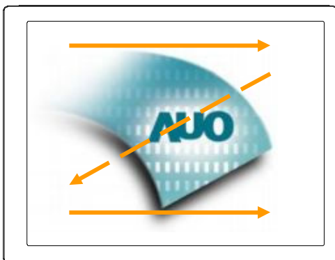
Fig. 1 Normal scan (Pin4, REV = Low or NC)
