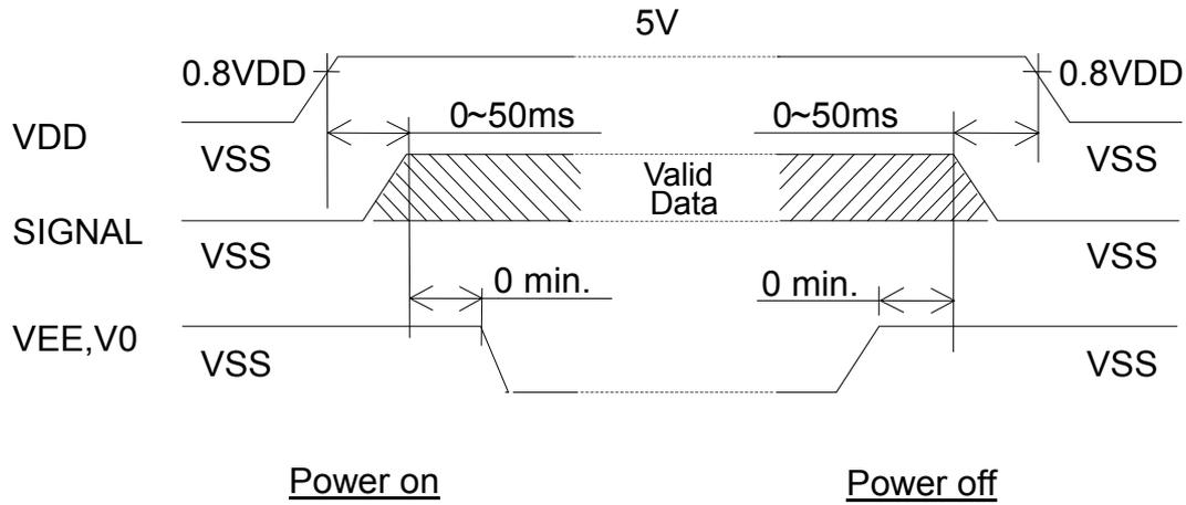
The missing pixels may occur when the LCM is driven beyond above power interface timing sequence.
